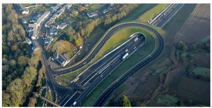
The scheme includes the construction of 16 major structures, over 12.5km of various types of retaining walls as well as excavation of over 1.3million m3 of earthworks. All this through an extremely narrow rock gorge whilst maintaining current traffic flows on the existing route.
