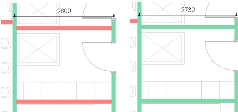
Figure 5 – ‘Before’ and ‘After’ images showing wall length reduction
