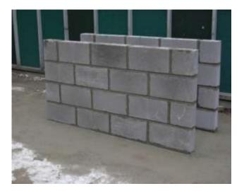
Figure 2 – Low-impact Portland cement-free building blocks and jointing mortar, developed at the University of South Wales to simulate typical products made using Portland Cement (Industrial Trials were carried out in collaboration with WD Lewis concrete block company at Aberdare, South Wales).
