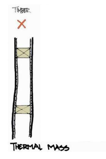
Timber - NO - Cellular construction – no heat retention
