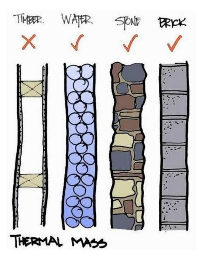
Timber - NO - Cellular construction – no heat retention
