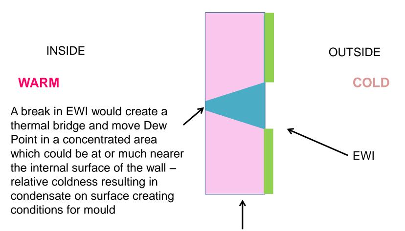
The location where saturation (Dew Point) could be somewhere within the thickness of the wall – where the temperature of the building fabric reaches a low enough temperature to create Dew Point
