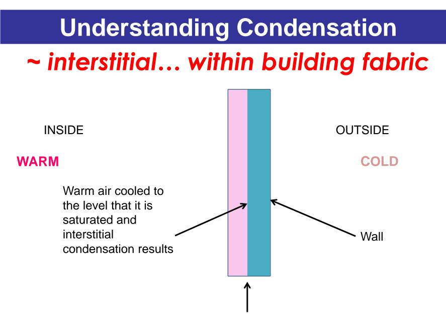
The location where saturation (Dew Point) could be somewhere within the thickness of the wall – where the temperature of the building fabric reaches a low enough temperature to create Dew Point
