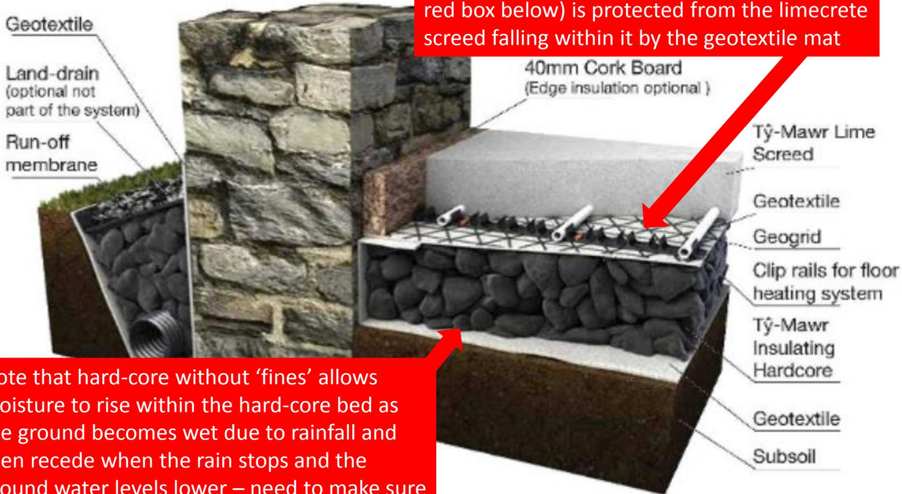
Note that the hard-core without 'fines' (see red box below) is protected from the limecrete screed falling within it by the geotextile mat
