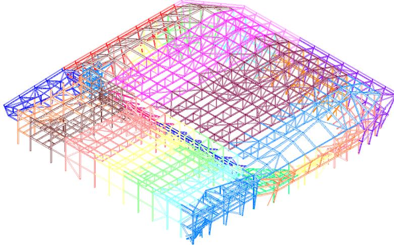
Figure 5 – Structural steel elements coloured based on the installation dates used for the deconstruction timeline
