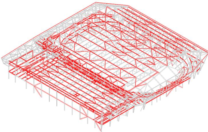
Figure 4 – Structural steel elements coloured red where there is a high grade of possible reuse.
