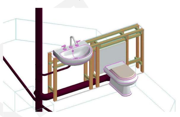
**Timber frame structure** The timber frame structure was made available as a 3D model. It was imported in the BIM model for clash detection with the architectural design.
