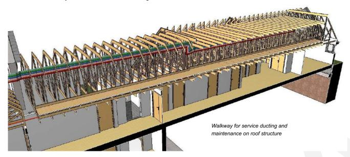
This is a valid strategy but to avoid waste of materials, time and workmanship it needs to be followed by a detailed 3D model of the proposed M&E systems that in its turn will be checked against the architectural design. Clash detection and case-by-case design can happen in advance ensuring the use of the best routes and more economical layouts.
