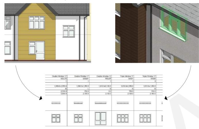
The technical specification for the construction elements were taken from the drawings provided and researched online. It was incremented or modified during the model construction and management.
