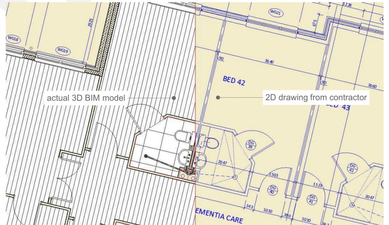
BIM objects were created to match the doors and windows types and easily populate the model. That also resulted in an automatic schedule of openings.
