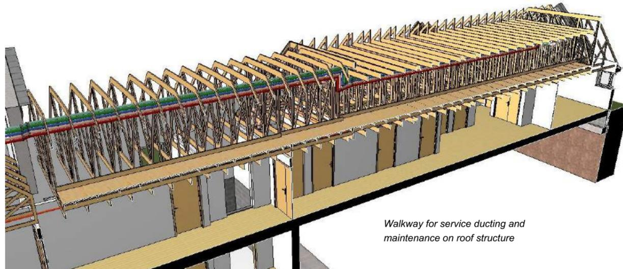
This is a valid strategy but to avoid waste of materials, time and workmanship it needs to be followed by a detailed 3D model of the proposed M&E systems that in its turn will be checked against the architectural design. Clash detection and case-by-case design can happen in advance ensuring the use of the best routes and more economical layouts.
