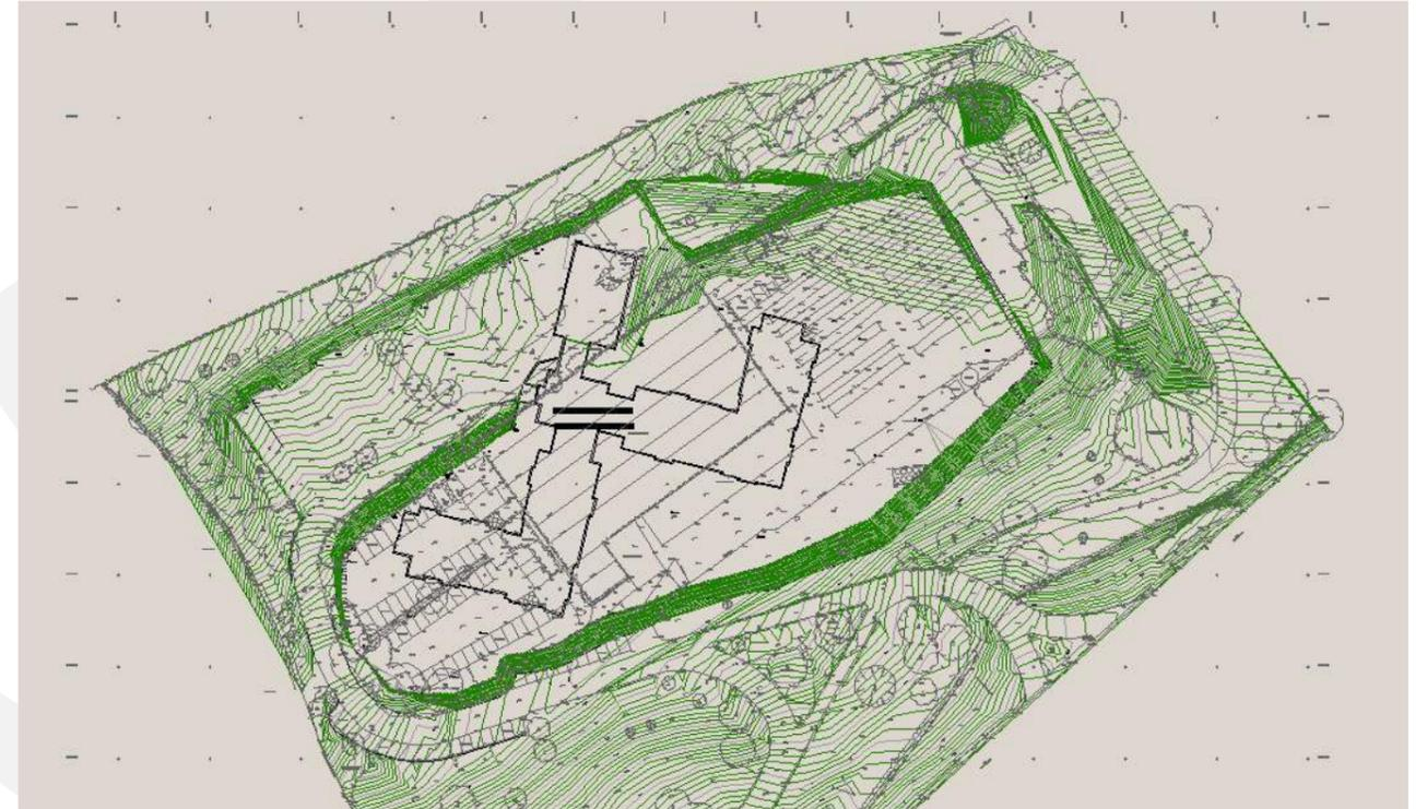
2D curves used as reference to model the terrain
