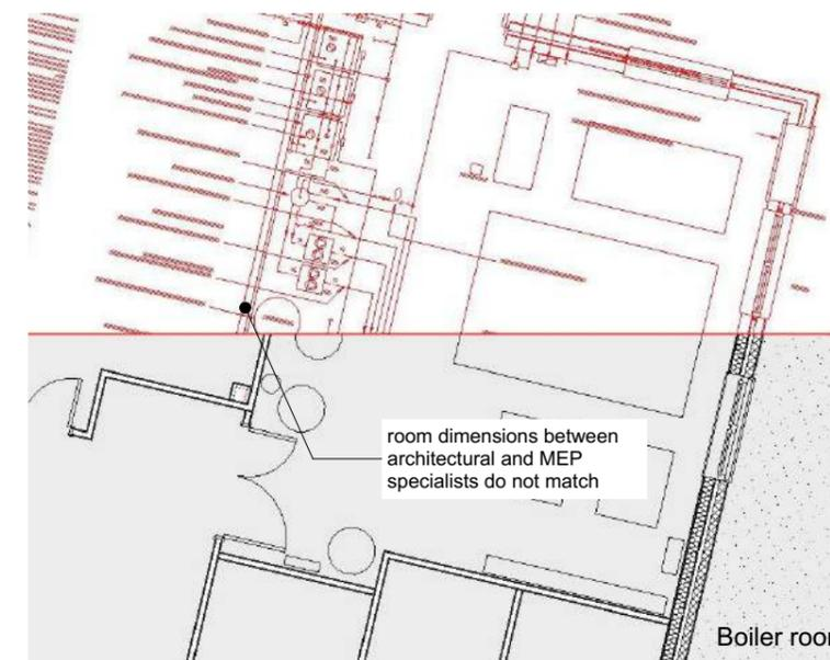
In this case there was a significant discrepancy between the dimensions of the boiler room as shown on the architectural and MEP specialist drawings. Such difference on the space allocated for machinery could have meant abortive work, rebuilding of walls and floors, and delays on the completion targets.
