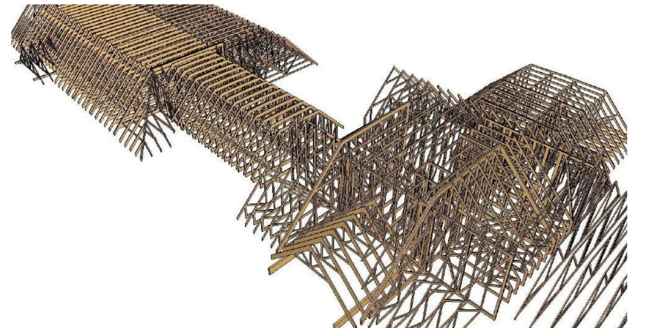
It was agreed (for the purpose of this exercise) that only a portion of the roof would be modelled to avoid excessive cost and time. For the purpose of this exercise, the parts of the building modelled were the technical block (containing the boiler room, kitchen, staff bathrooms and toilets, and the laundry) plus the entrance hall.
