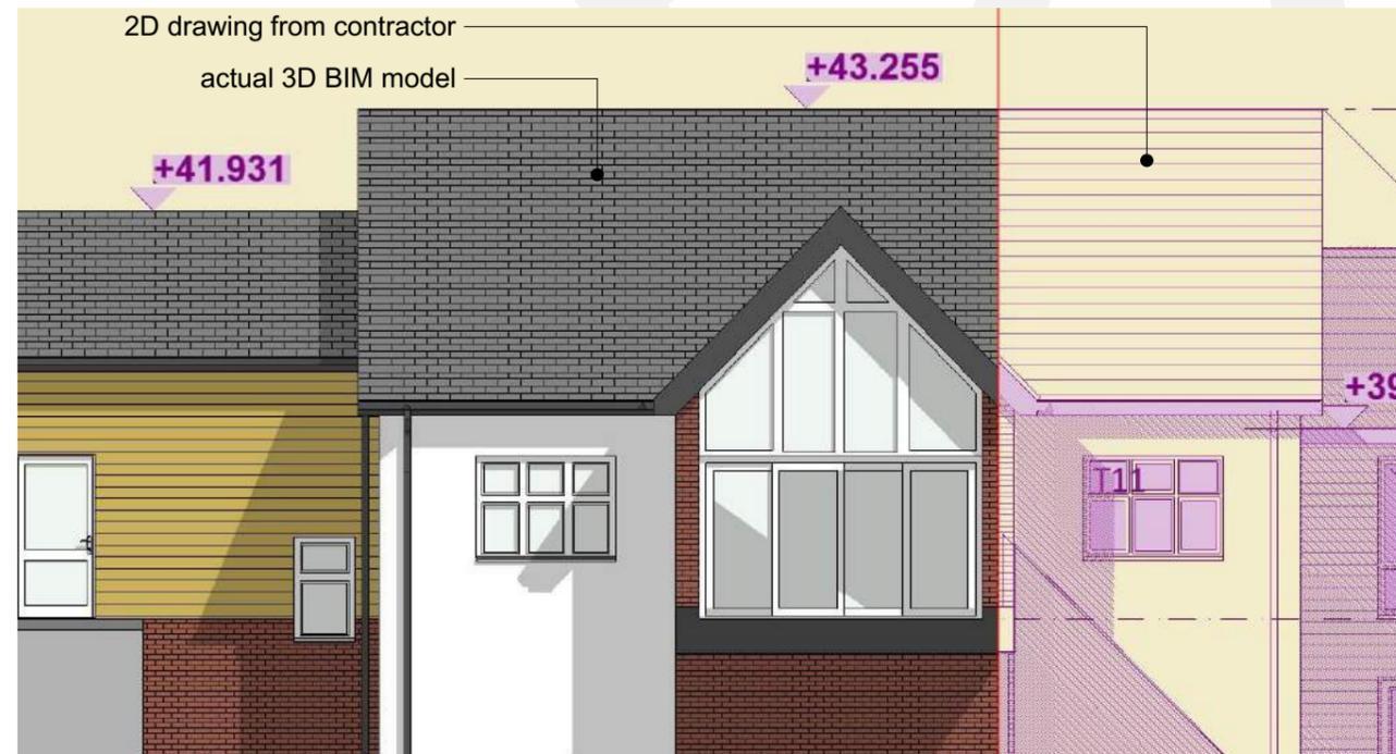
Differences between the roof levels in the plans and elevations were identified. To make the roof geometry match in 3D, small adjustments in the roof angles would be necessary, departing from the 45 degrees indicate in the drawings.
