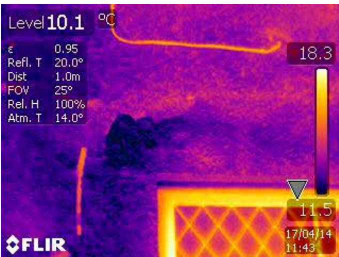
Figure 27: Cold Bridge introduced at area of spalled render.
